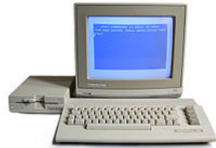
Commodore 64c with 1541-II floppy disk drive and 1084S monitor displaying television-compatible S-video
