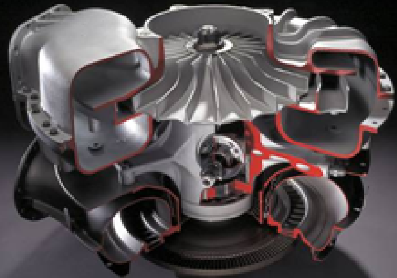
Type C-Series Turbosupercharger Cutaway General Electric
