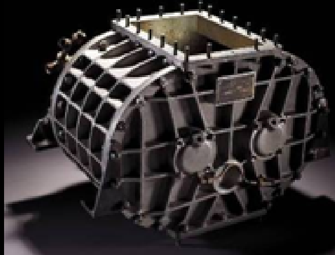
Type C-Series Turbosupercharger Cutaway General Electric
