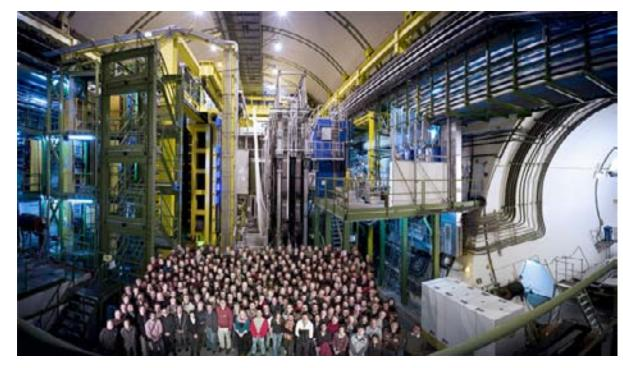
Size: 21m long, 10m high and 13m wide Weight: 5600 tonnes Design: forward spectrometer with planar detectors Location: Ferney-Voltaire, France.
